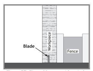
**Figure 57.** First rabbet cut with a single blade.
